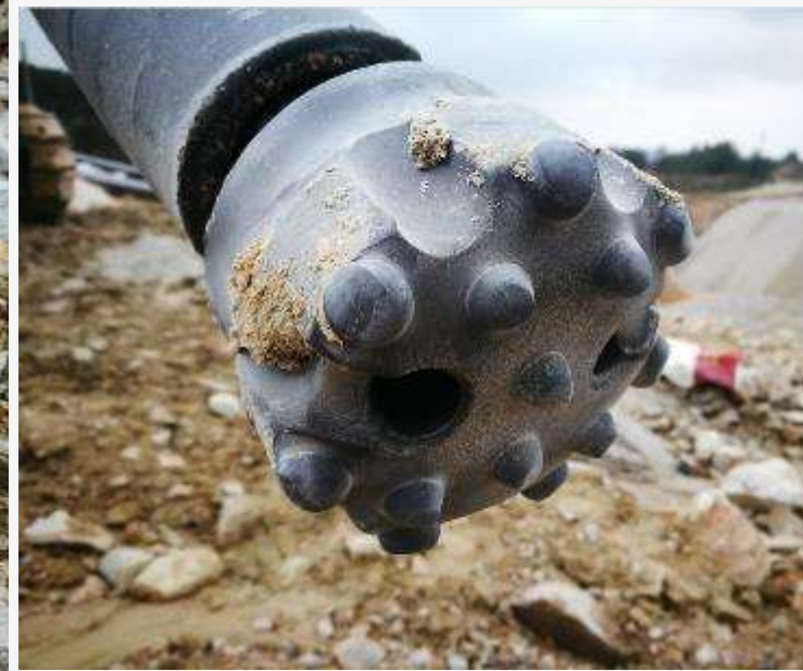
2019, Dec, in Hunan Province, Changsha xiangjiang quarry KD05 Carbide buttons in DTH BITS
